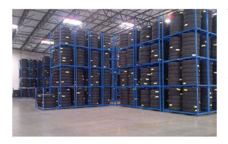
This system is durable, portable, collapsible, shippable, low-cost, stacking racks that reduces costly product damage associated with bulk stacking, offers better space utilization, product identification and easier handling of product.
