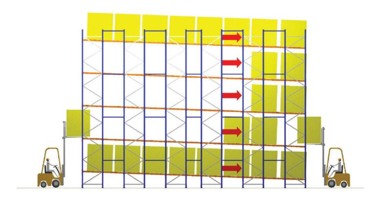
Flow rack is also called pallet flow racking, whose rollers are fixed up in the beam of the shelf at a fixed gradient and then palce the pallet in the higher side, so it will be fallen depending on its own gravitation. In order to control the pallet in a steady speed and avoid the collision, a set of damping system will be set up on the roller line at every certain distance since the faster speed pallet slide, the more the resistance that damped system caused.
