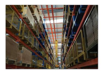
Automated storage and retrieval systems, sometimes known as ASRS or AS/RS, are made of a variation of computer-controlled systems that automatically place and retrieve loads from set storage locations in the store with precision and speed.
